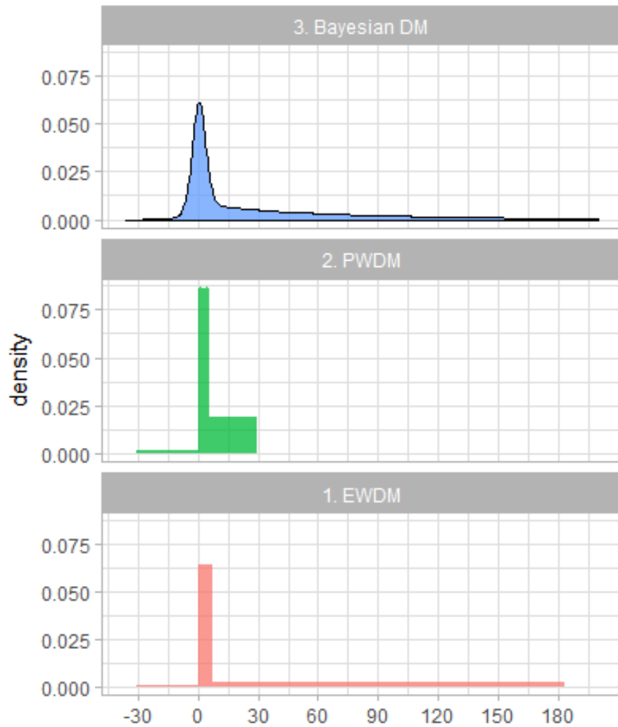
Figure 7.15: Final distributions for target variable 10: ‘What is the typical gap between major gas outburst episodes?’ Note, similar to the PWDM (although not the same extent) the Bayesian DM puts more of the distributional density in the region just greater than the modal point. Whilst the Bayesian model includes the greater range suggested by the EWDM it tapers off much faster.
