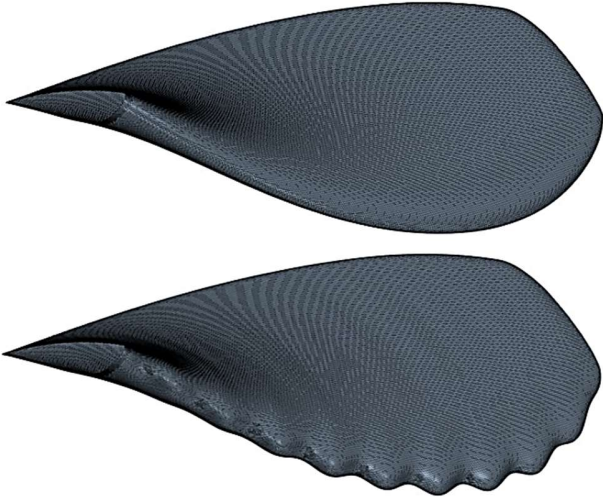
FIGURE 5: THE BASE AND TUB BLADE SURFACE MESH
