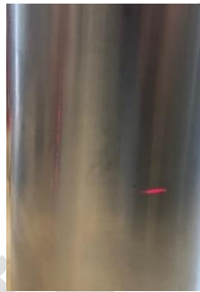
Fig. 5 Laser dots on the aluminum sample when the laser yaw angle was tilted. The laser dot lost its integrity and was spread as a line.
