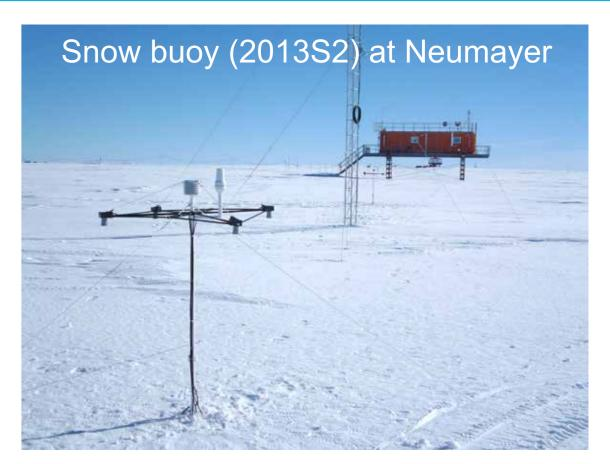
We developed a new buoy type to obtain time series of snow depth and air temperature on Arctic and Antarctic sea ice. The buoy is based on four sonic ranging sensors, and transmits the data via Iridium satellites.
