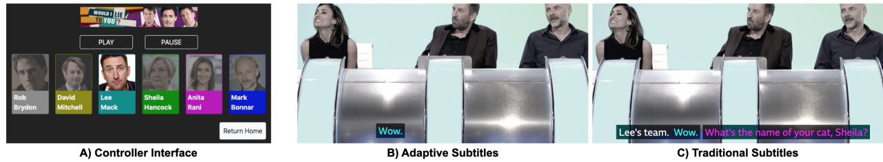
Figure 1: A) Adaptive Subtitles ‘Controller’ interface displaying speakers for BBC’s ‘Would I Lie To You?’ clip; Lee Mack has been toggled to have subtitles displayed. B) Adaptive Subtitles displaying subtitles for speakers selected in A. C) Traditional subtitles showing dialogue for all speakers.
