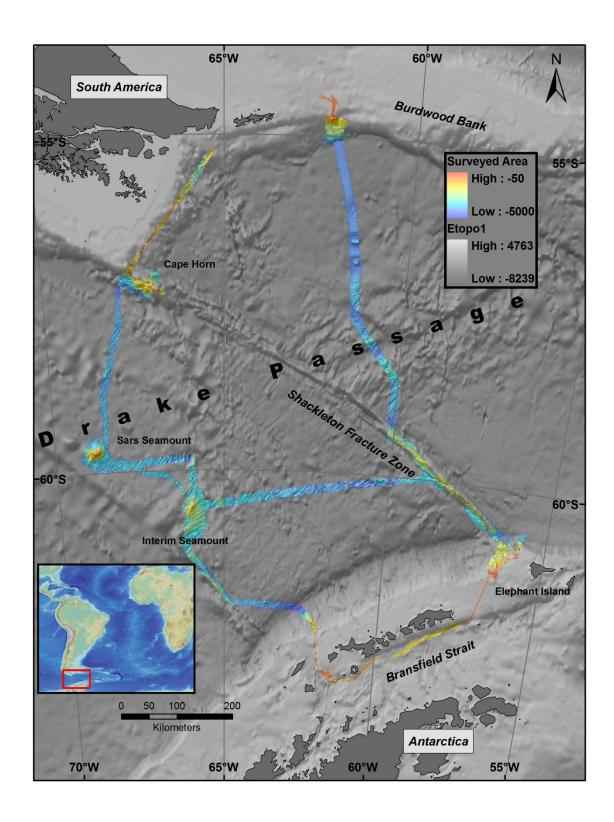
Figure 1: Location map showing multibeam bathymetry coverages from cruise NBP1103 and the portion of cruise NBP0805 that was in the Drake Passage.
