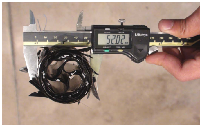
Figure 3.23: Model C1 packaged to a diameter of 52 mm.
