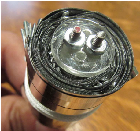
Figure 2.15: Model A2 wrapped around the guides. The packaged diameter was 23.9 mm.
