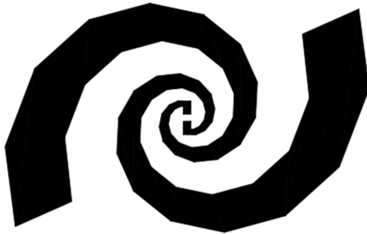
Fig. 60. Tu's spiral antenna fed perpendicularly by co-planar strip line.
