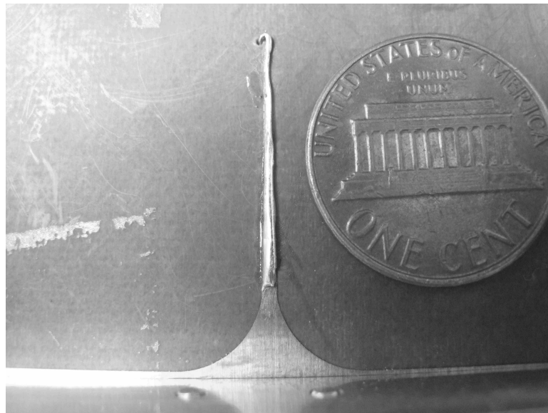
Fig. 5. Tapered parallel-strip line feed for the modified spiral.
