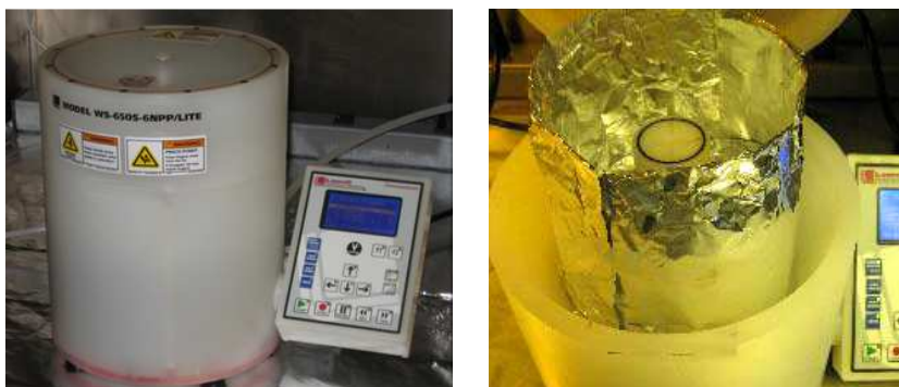
(a) (b) Figure B-2. (a) Spin Processor, and (b) Covered Stationary Seal
