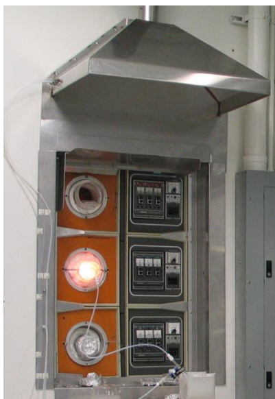
Figure 3.7. Photograph of a diffusion furnace used for thermal anneal of APE waveguides.
