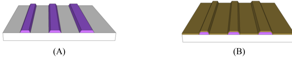
Figure 4.2. Incorrect resist profile for lift-off. A) Positive resist, when developed has a slightly obtuse edge profile. B) The obtuse profile, when sputter coated, creates a solid blanket layer of material which isolates the resist, impeding the lift-off process.
