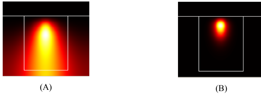
Figure 2.15. These figures are for the mode propagation simulation of an APE waveguide fabricated with initial exchange 20min@200C, and subsequently annealed for 4 hours at 400C. The images depict the two dimensional mode profile as found with FimmWave waveguide modeling software. A) Simulation using Almeida's refractive index relation. B) Simulation using Pissaro's refractive index relation.
