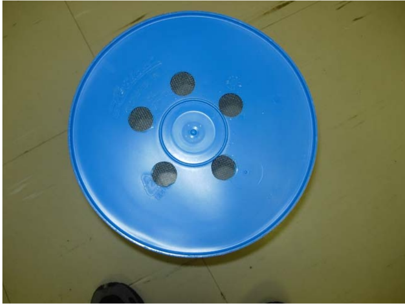
Fig. 6. A 19 L bucket with five 2.54 cm holes with fiberglass window screen in place to hold soil.
