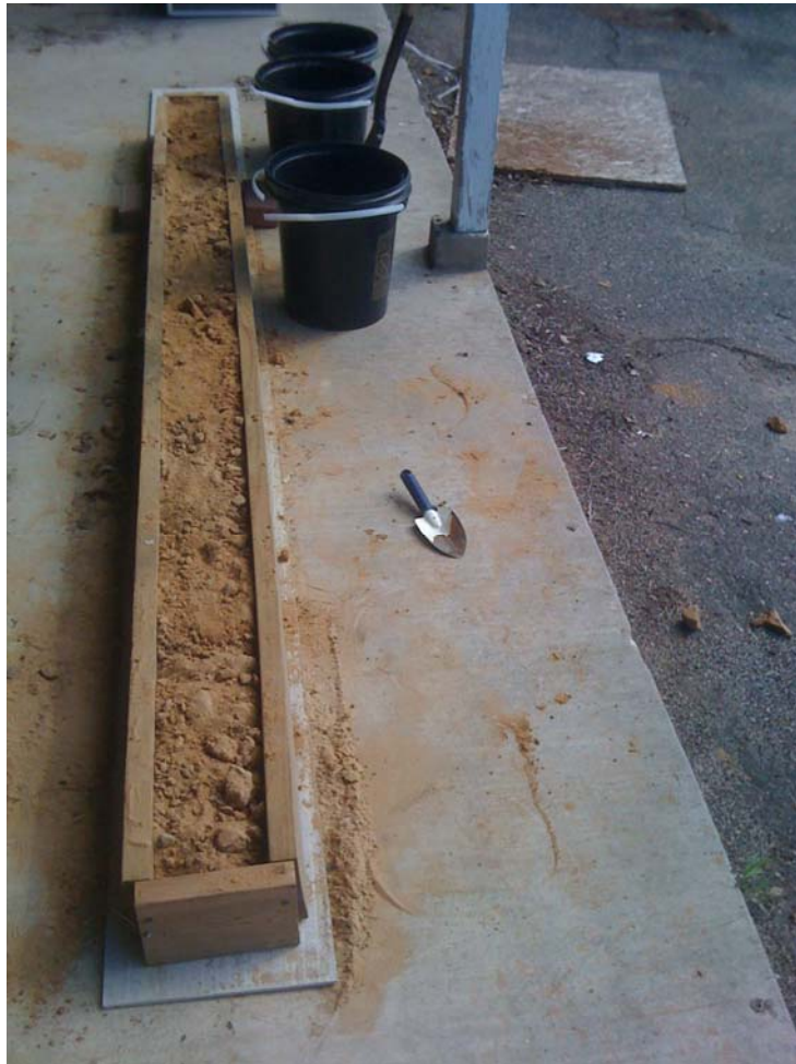
Fig. 7. Simulated trench with the following specifications, 3.05 m long by 15.24 cm wide and 15.24 cm deep.
