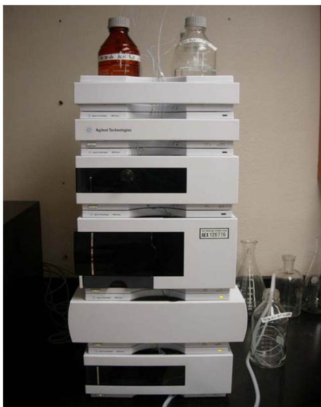
Fig. 2. HPLC with all components: solvent cabinet, vacuum degasser, quaternary pump, autosampler, column compartment, and diode array detector (DAD).
