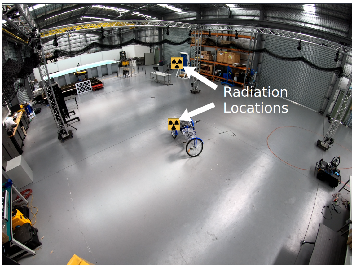
Figure 5. Photograph of indoor test environment 2, highlighting radiation source locations.
