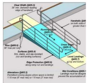
Figure Ramp Requirements [§405] Gambar Persyaratan Bidang Miring [§405]
