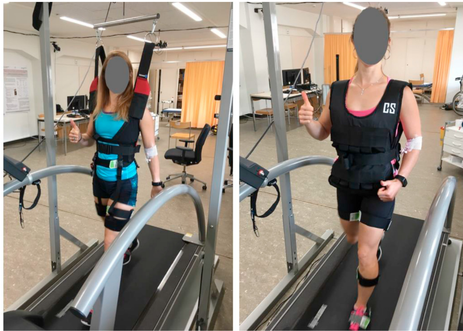
Fig. 1. Left: participant walking in the reduced load condition with a 20% dynamical reduction in bodyweight. Right: participant walking in the increased load condition with increase in bodyweight corresponding to 20% body mass.
