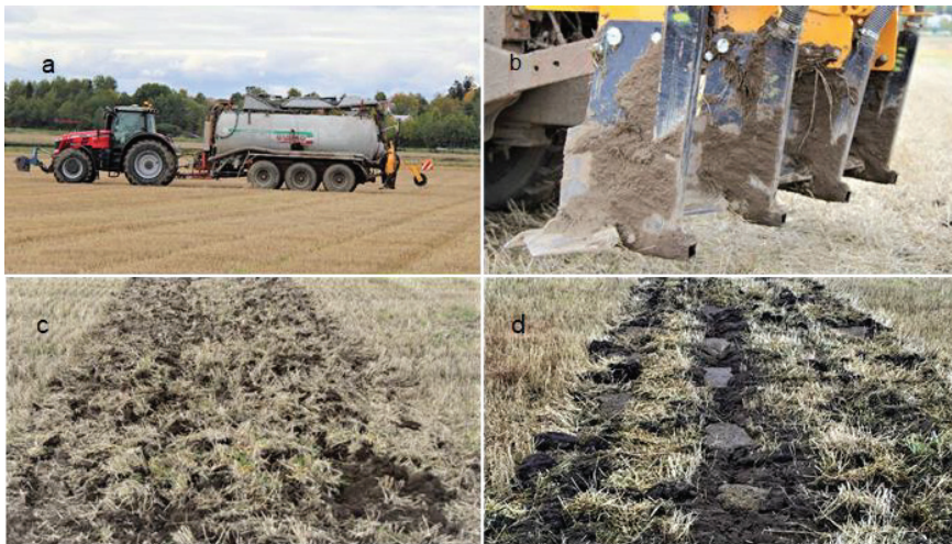
Figure 1. a) Subsoil loosener being drawn behind the tanker containing straw slurry, b) close-up view of the modified subsoiler with metal channels, c) soil after subsoil loosening, and d) soil after subsoil loosening with straw slurry addition.
