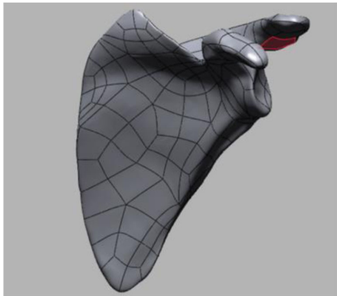
Fig. 5 Surface generated by Geomagic Design X associated with the scapula
