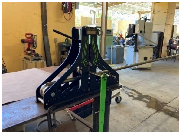
Figure 6.3. Tubing roller "Hulk" with pipe set up between pinions.
