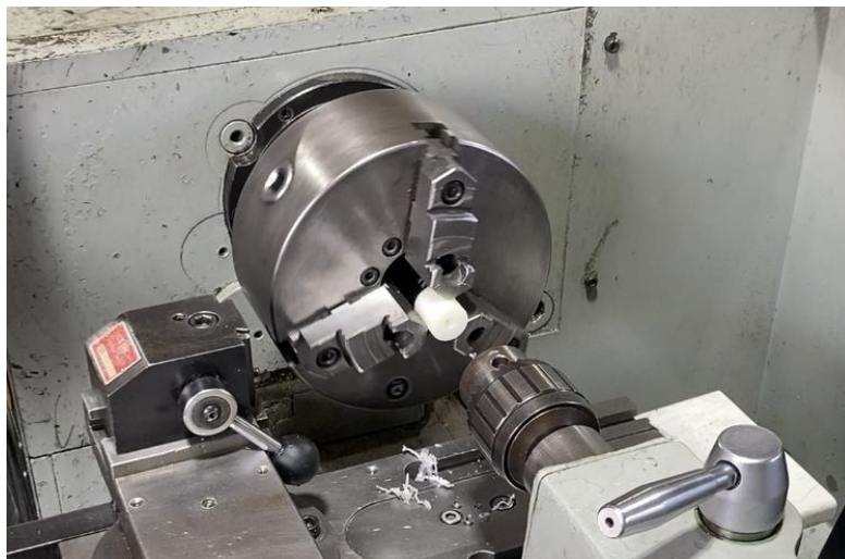
Figure 6.1. Drilling pilot hole in nylon stock.
