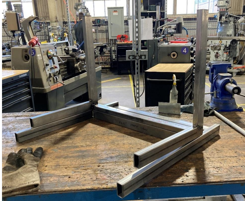
Figure 6.6. Partially completed frame and forks.
