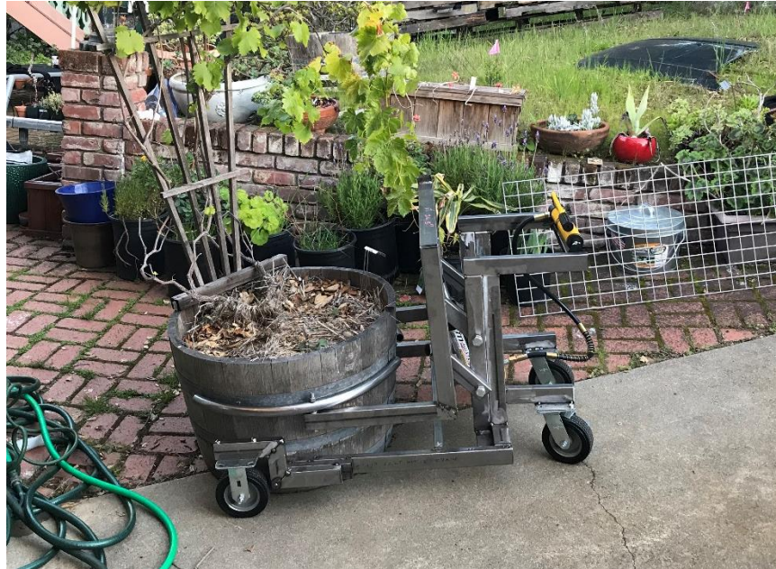
Figure 9.1. Completed verification prototype holding barrel planter.
