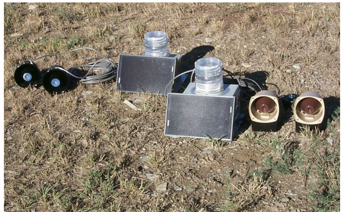
Figure 8. A Radio-Activated Guard (RAG) box consisting of a radio-telemetry receiver that activates the unit when a radio-collared wolf is detected. Unit consists of strobe lights, solar-powered battery, user defined activation distance, and plays more than 30 different sounds to scare the wolf away.
