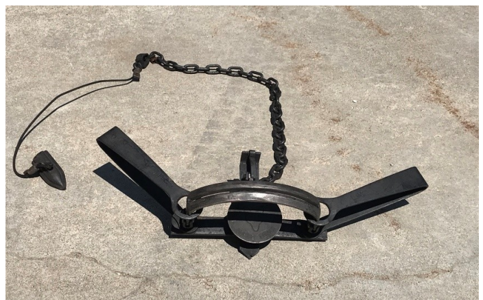
Figure 13. Foothold trap equipped with a “bullet” anchor which is driven into the ground. When the chain is pulled, the anchor pivots, anchoring the trap in place.
