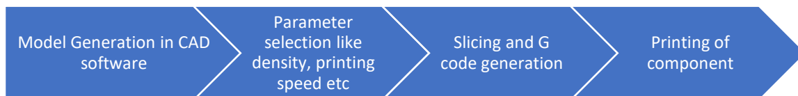
Fig 1: General process of 3D printing
