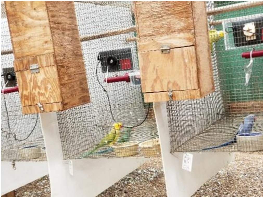
Figure 2.1 Tablet and delivery system equipment setup in caging. Rose-ringed parakeets at a commercial aviary near Austin, Texas. Birds are visually separated with an opaque barrier between cages. The black tablets, mounted inside the cage in bird-proof boxes, connect to the maroon colored delivery device. A plastic funnel (pulled out for photograph, rightmost cage), delivers items from the tablet system into the food dish. The birds' nest boxes are visible on the front of the caging.
