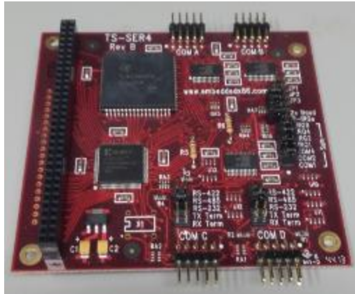
Figure 38: TS-SER4 Serial Expansion Board
