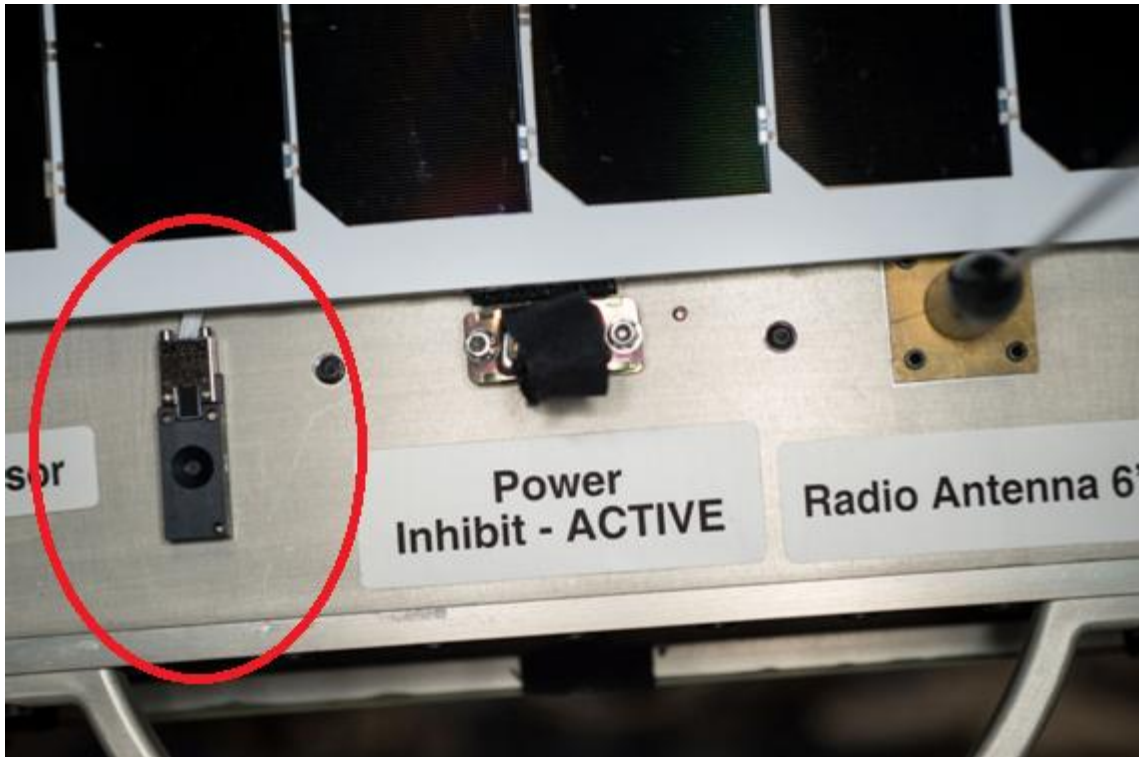
Figure 66: Sun Sensor Installed
