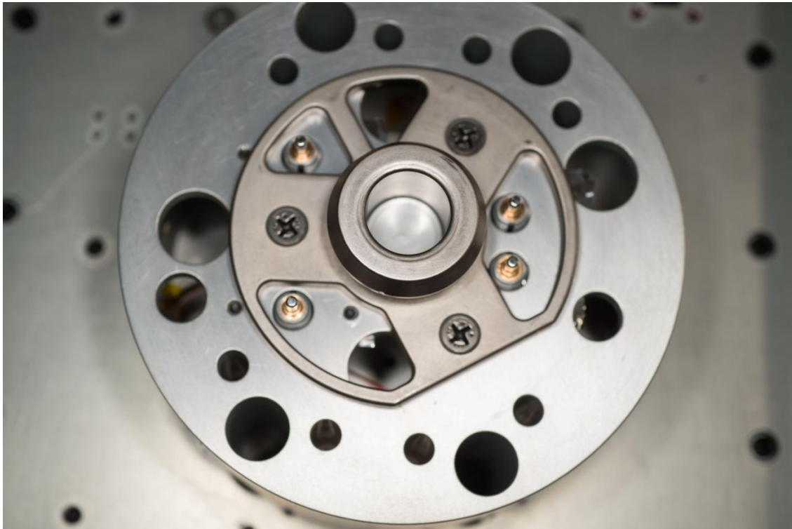
Figure 83: Cyclops EAF and Inhibit Switches
