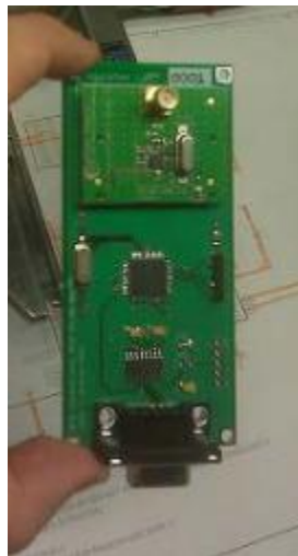
Figure 60: HDR Radio Unit Design (photo by Graves, Dec. 2011)
