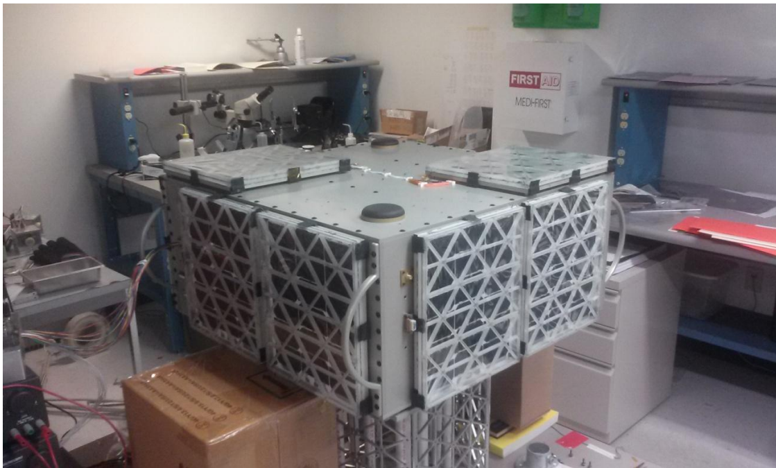
Figure 91: Bus with Solar Panels and Covers Installed
