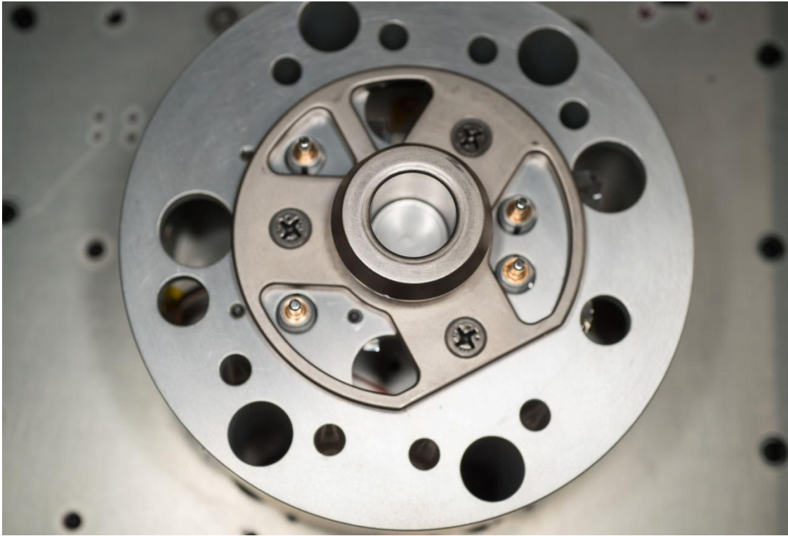
Figure 56: AGS4 Inhibit Switches
