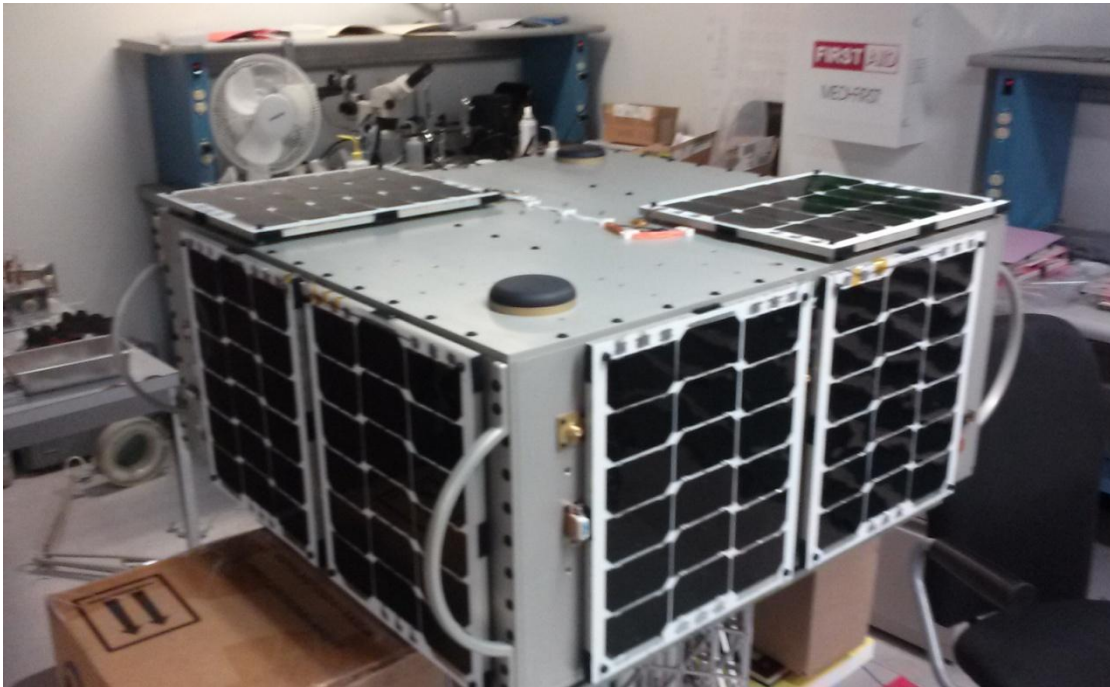
Figure 53: Top and Side Solar Panel Configuration
