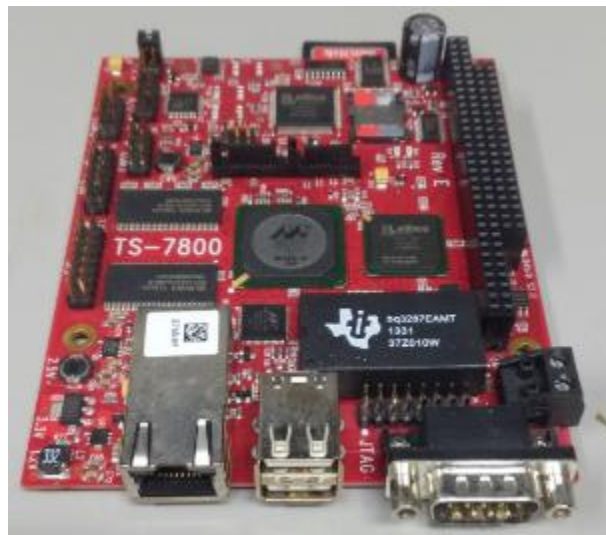
Figure 37: TS-7800 Flight Computer
