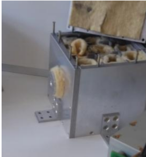
Figure 50: Battery Box Vent and Cover
