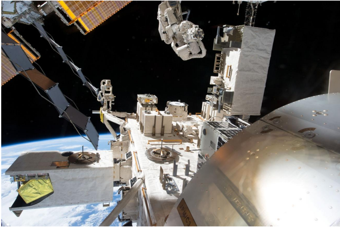
Figure 106: AGS4 and Cyclops Table Moved onto Porch (Photo by NASA)
