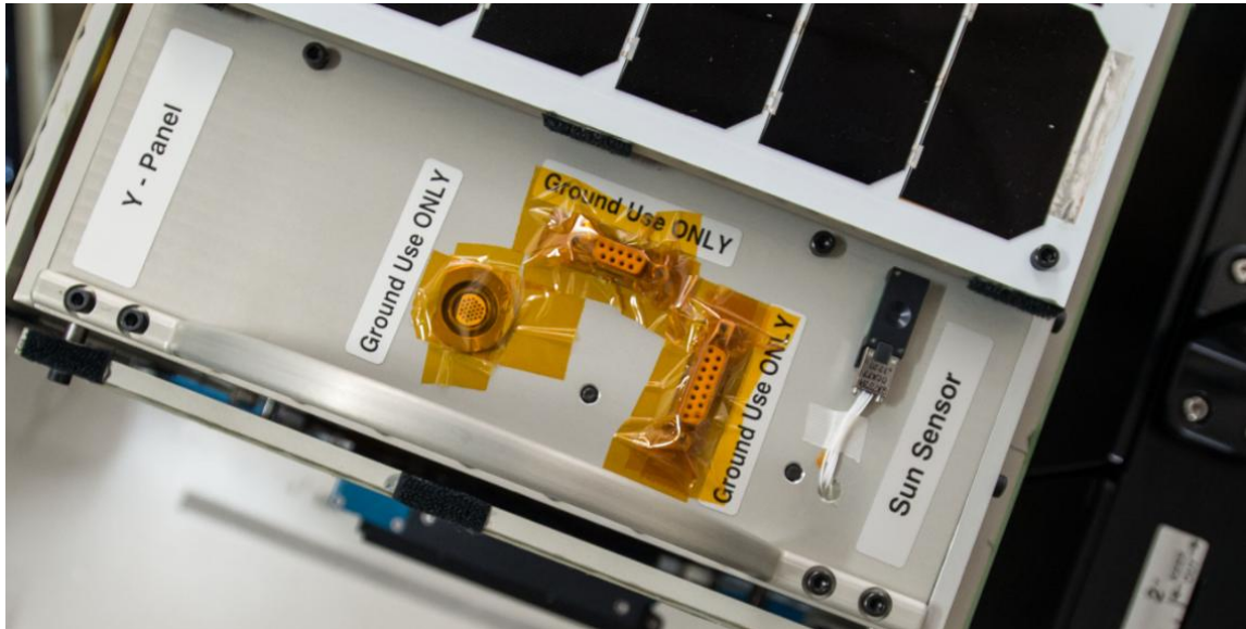
Figure 96: Computer Access Ports for AGS4 (Circular) and Bevo-2 (DB-9/DB-15)
