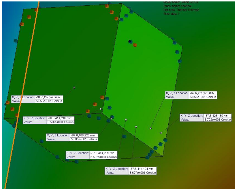
Figure 112: Battery Box Thermal Analysis Probing
