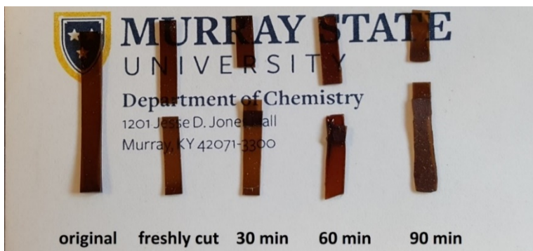
Figure 2.3: Samples from a representative re-heal stress-strain trial for PIL-CAN-IM2 at 105 °C. From left-to-right: original sample, freshly cut sample, 30 min re-heal sample, 60 min re-heal sample, 90 min re-heal sample.
