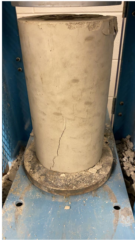
Figure 4. 10: Concrete Cylinder after Compression test
