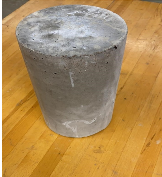
Figure 4. 8: Preparing Cylinder Specimens
