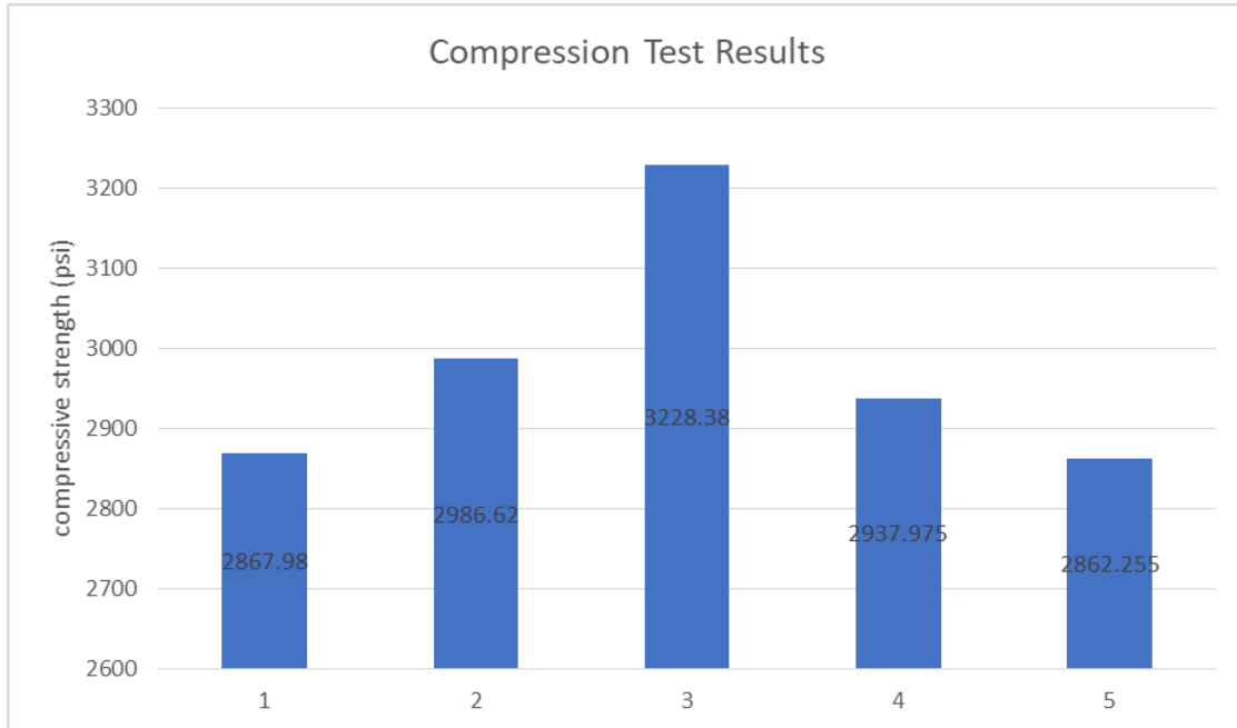
Figure 4. 6: Graphical representation of Tabulated Average Compressive strength
