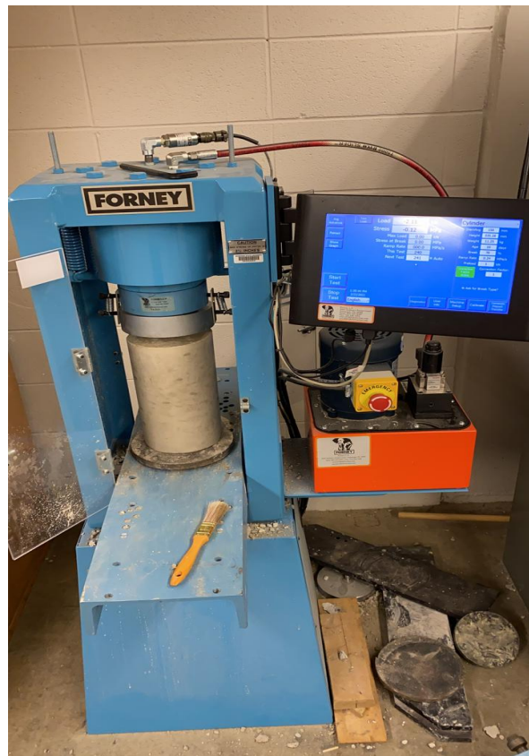
Figure 4. 9: Compression test of Cast Cylinders
