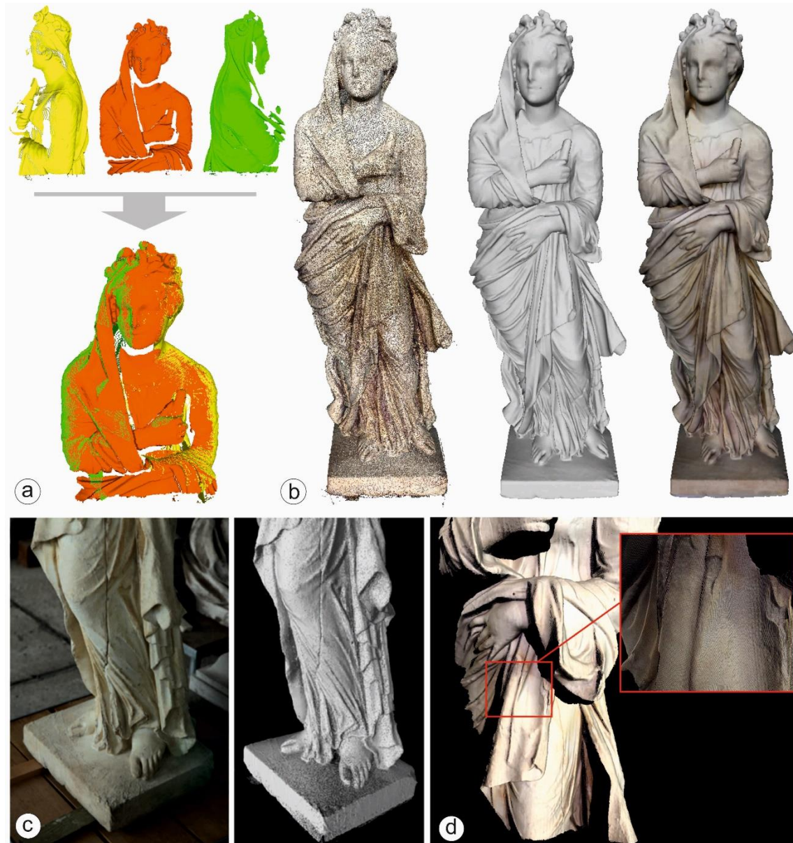
Figure 98 Steps to generate complete reconstructions from multiple views. (a) Alignment of partial point clouds. (b) Point cloud, mesh and textured mesh of the reconstruction. (c) and (d) show how the high-resolution reconstructions can document even small damages in the object's surface (Images were contributed by Fetzer, T.).
