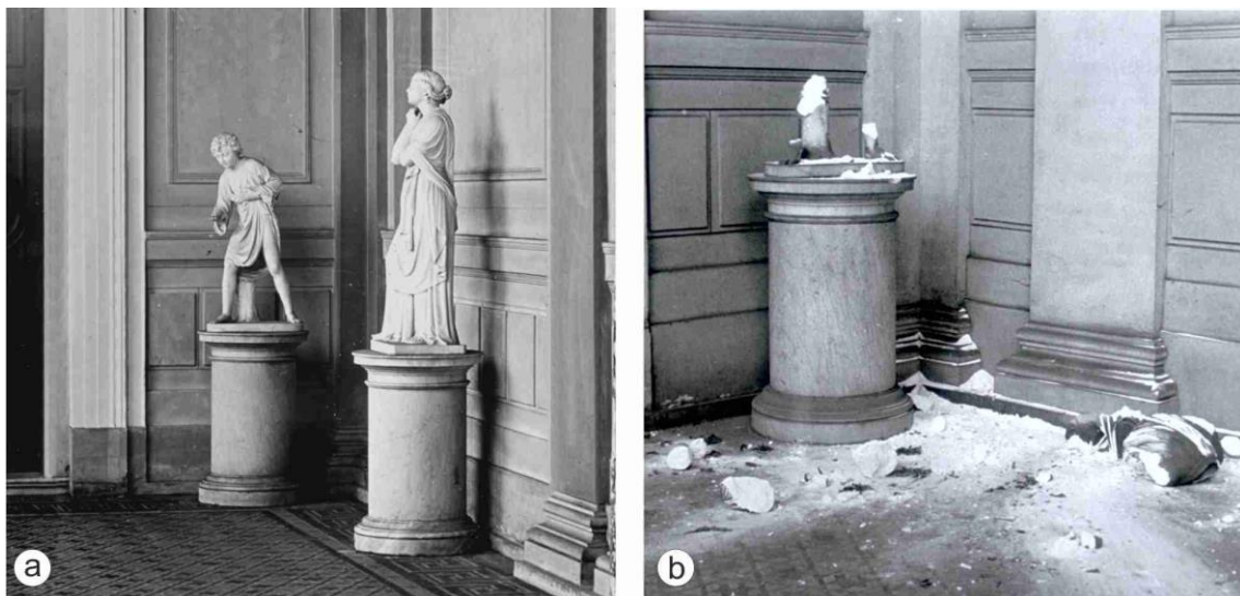
Figure 1 a) Sculpture in the Orangery, Potsdam, before total structural collapse in 1978 and b) after complete collapse after 110 years of exposure (modified after Siegesmund et al., 2004a).
