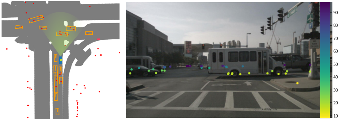
Figure 1.1: This figure shows the radar measurements from nuScenes dataset [1]. The left image is the bird view of the scene. The ego vehicle is indicated using a patched blue rectangle, radar measurements are plotted by red points, and the annotated vehicles are orange rectangles. The right figure overlays the radar measurements on the camera image with colors indicating depth.
