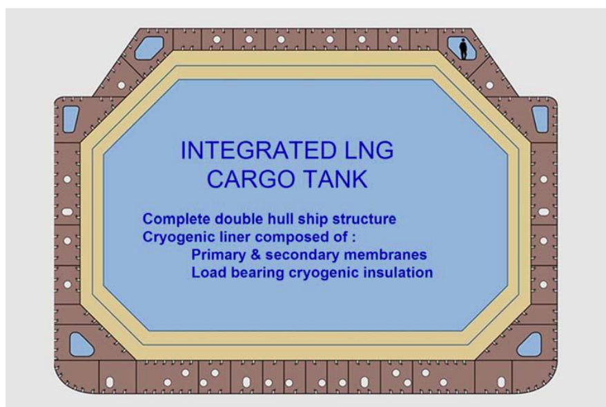
Figure 5-Generic Membrane Tank Source: DNV, 2011b
