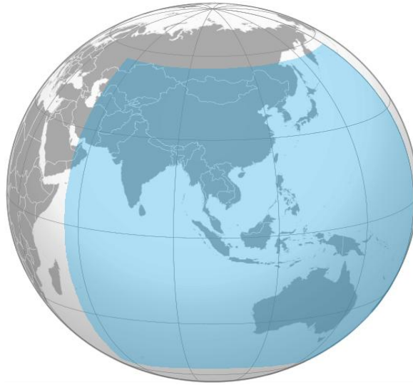
Figure 2.18 BDS service coverage area (Source: www.beidou.org.cn )
