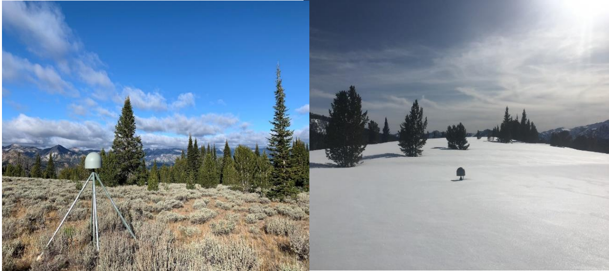
Figure 3: GNSS station P360 at Galena, Idaho, during summer (left) and winter (right). The station is deployed on a flat surface. In winter the antenna is not completely buried by snowpack, so there is no loss of data.
