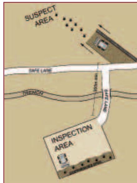
Fig. 19. Suggested positioning of inspection area in relation to suspect area
