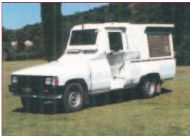
Fig. 23. An example of a V-shaped capsule mounted on the chassis of a light commercial vehicle
