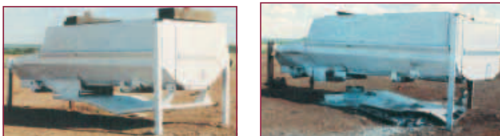
Fig. 27. Effect of a SFF test mine on a capture plate fitted underneath the hull of a MPV capsule
