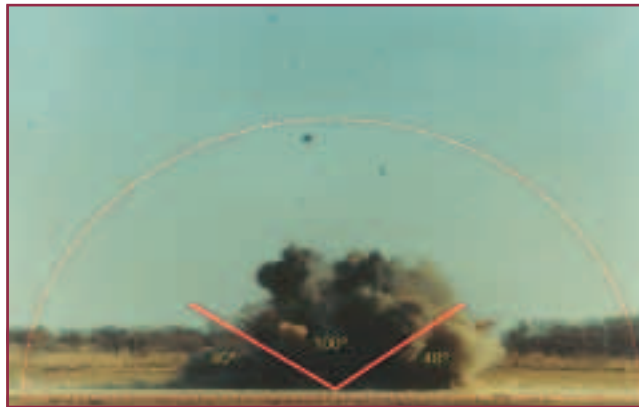
Fig. 6. Final development of explosive shock wave approximately 5 milliseconds after initiation of a 7 kilogram TNT test charge buried 100 millimetres under the surface.
