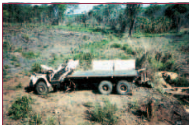
Fig. 9. Unprotected medium-sized vehicle that detonated a single anti-tank mine under the right front wheel
