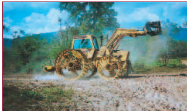
Fig. 30. Pearson Engineering SDTT. The Pearson Roller is attached to the tractor. Used in Thailand.
