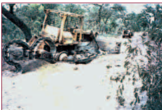
Fig. 10. Bulldozer after detonating a single TMA 3 mine in Mozambique
