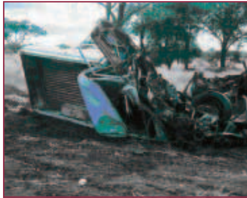
Fig. 8. Light unprotected pick-up destroyed by the blast from a single TM 46 anti-tank mine under the left front wheel
