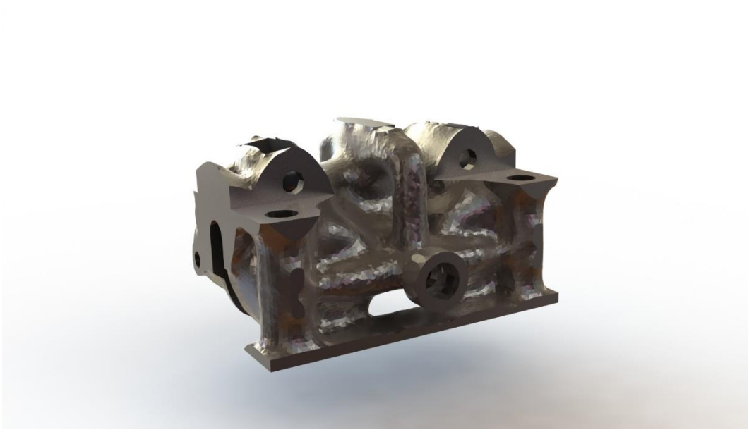
Figure 20: Side profile of brake caliper after topology study
