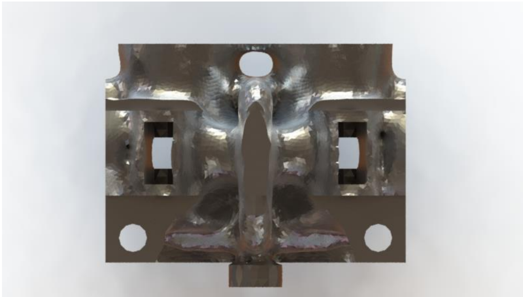
Figure 21: Top profile of brake caliper after topology study
