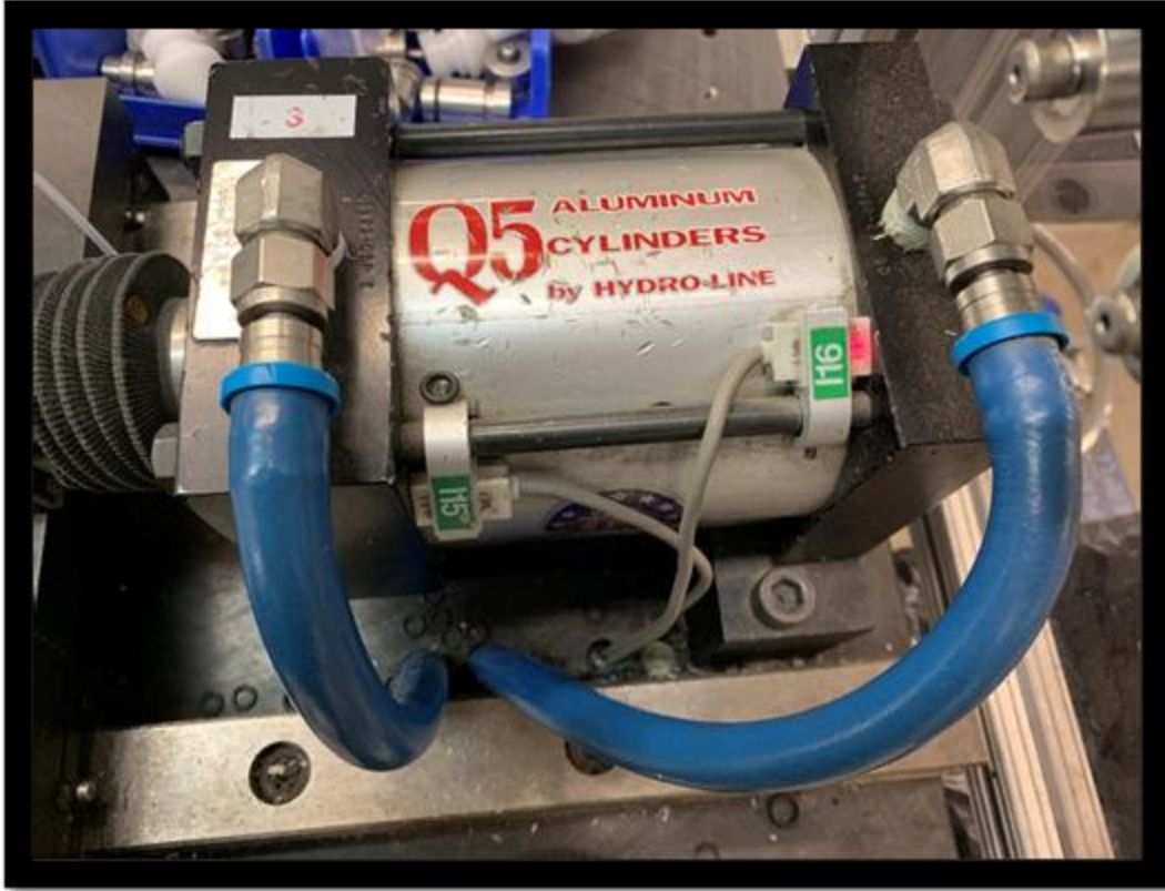
Original Air Cylinder with barbed push in style connecting hose.
