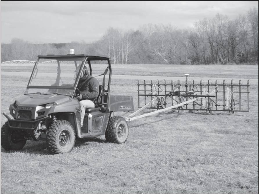
Figure 2. SENSYS Magneto ® MX v3 magnetometer system in action. (Photo R. Komp (DAI))
