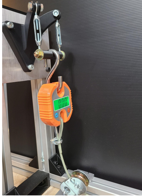
Figure 18: Test Bench with Unoptimized ABS Part Attached
