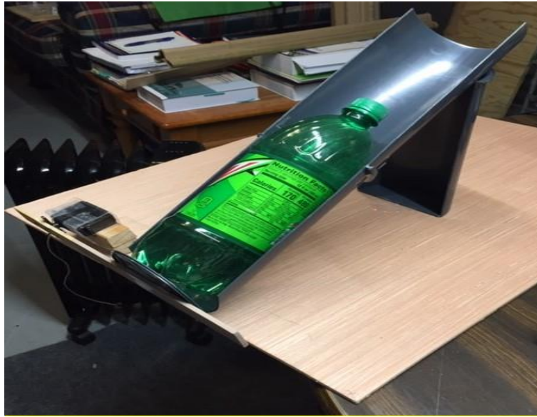
Figure 6.3.2: Detection Area/Load Cell Top Mock-up (KRS)
