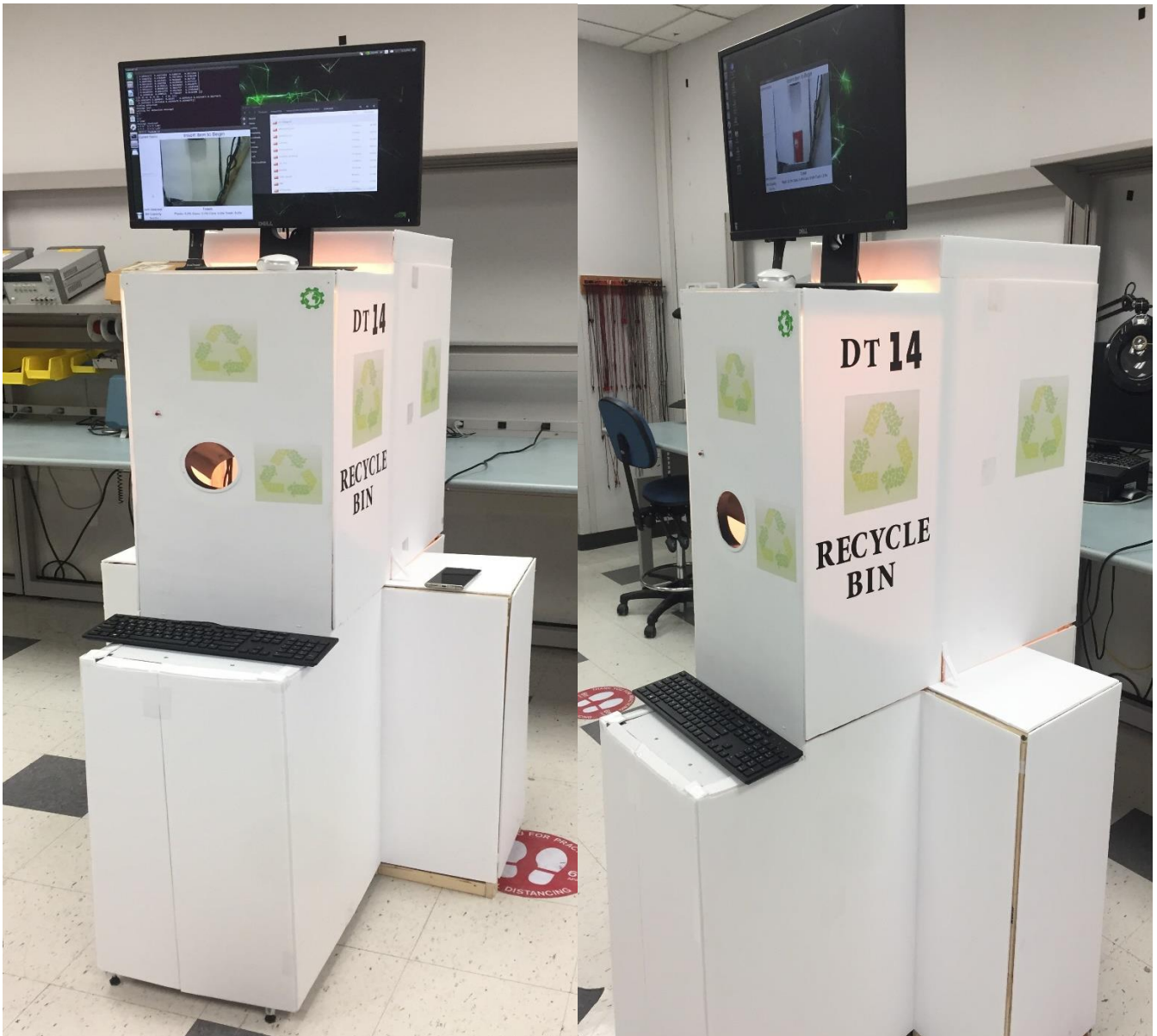
Figure 6.4.4: Completed and Enclosed Smart Recycling Bin (KRS)
