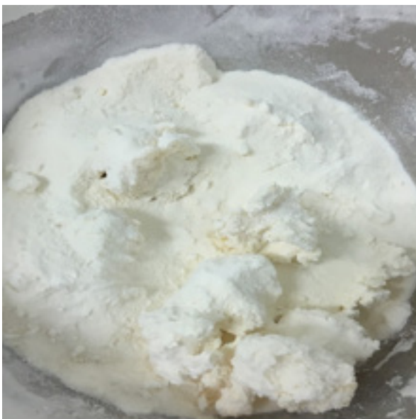
Figure 3. A representative image of agglomerated powder produced in treatment that had the combination of 140 g of pre-wet mass and 5.6 mL/min flow rate. The resultant powder did not meet the industrial specification of whey protein isolate.
