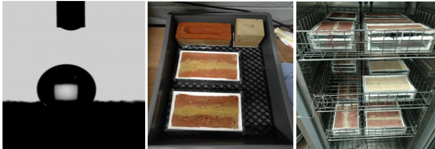
Figure 1: a) Water drop on treated specimen, b) 3 different types of specimen used for absorption test, c) Arrangement of specimens for vapour transmission test.
