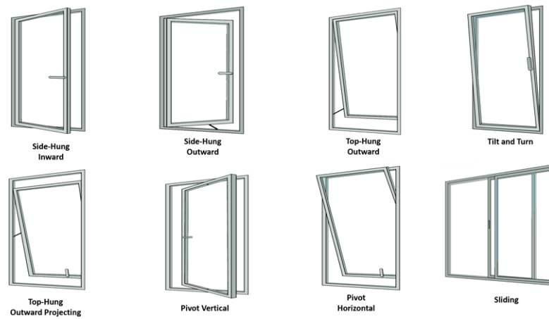
Figure 2.10: Typical PBSA window opening types (HNS, 2020)
