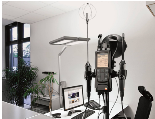
Figure 2.7: Example of equipment required for comprehensive indoor comfort assessment (Testo, 2020)
