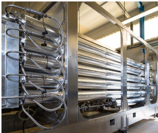
Figure 3.5 - Picture of the continuous oscillatory baffled reactor (COBR) developed by Arkema at GRL facilities in Lacq.
