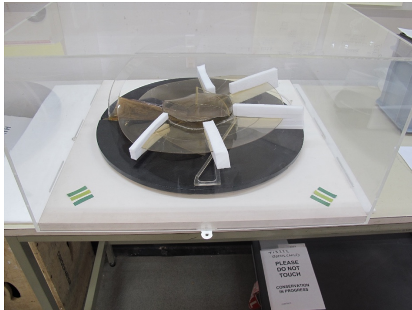
Figure 8-8 – A view of T02142 showing its placement on its bench along with the clear plastic cover over it. The sensor and SPME fibre were placed through cutouts on the bottom left of the plastic cover.
