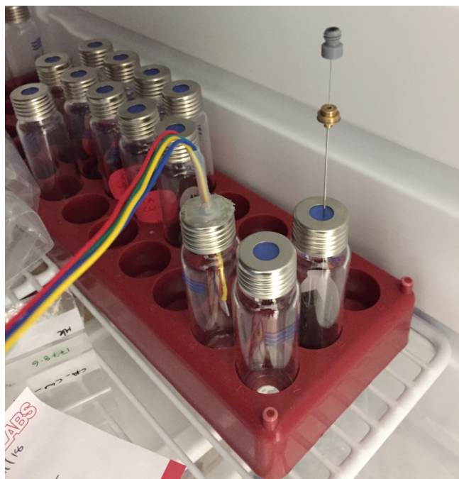
Figure 6-2 – Exposure setup inside the fridge during the experiment. This shows the vial which contained a temperature and relative humidity sensor along with a vial which has a SPME fibre placed inside it.
