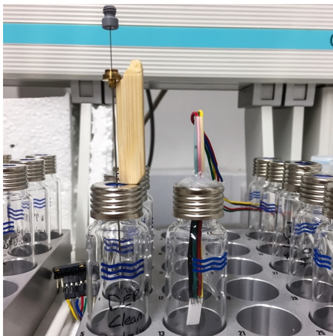
Figure 6-3 –Exposure setup for both 25 °C and 20 °C. To the left of the vial with a SPME fibre is a T/RH sensor which is monitoring the GC/MS area. Next to this is a vial which contains a sample. Also shown here is the larger of the two wooden depth markers. To the right of this is the vial containing another T/RH sensor.
