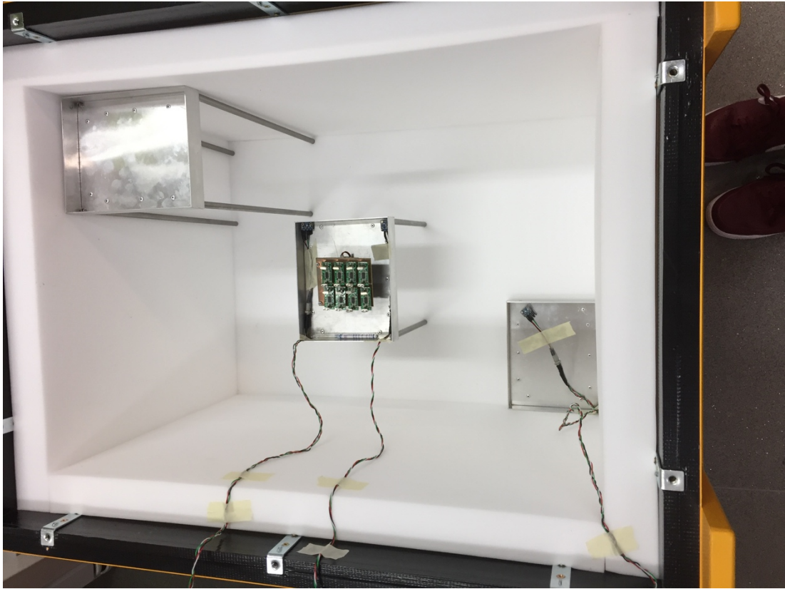
Figure 8-2 - Image of the three levels inside the crate. The levels were constructed from aluminium sheets and the bottom layer (on the right of this image) had no struts and was placed on top of the Plastazote. Note that the wires from the sensors were forced into the Plastazote when the crate cover was placed on top and as such the seal was not compromised.
