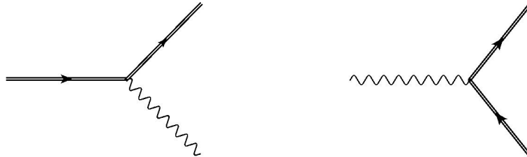
Fig. 1: Left: Nonlinear Compton scattering (photon emission). Right: Nonlinear Breit–Wheeler pair production. Double lines denote laser dressed (Volkov) electrons.
