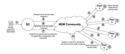
Figure 6: M2M Application Configuration
