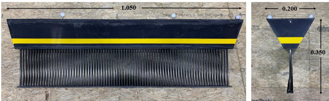
Figure 20. The windward side (left) of the pipe model design and the profile view (right) with waves propagating left to right. The top of the yellow line is the design water line. Dimensions are model scale and in meters.
