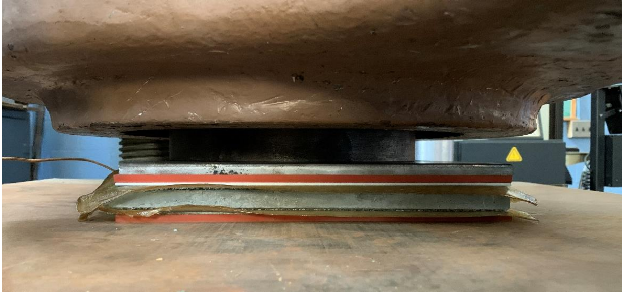
Figure 13: UHPC-thermoplastic sandwich panel undergoing consolidation.
