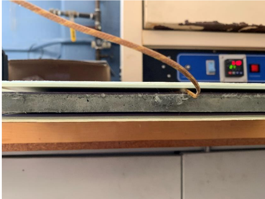
Figure 10: Thermocouple wire inserted between layup and adhesive layers.
