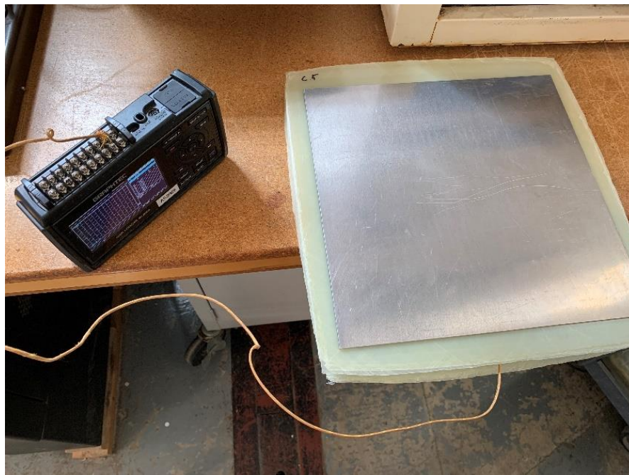
Figure 11: Thermocouple wire set up to panel prior to heating.
