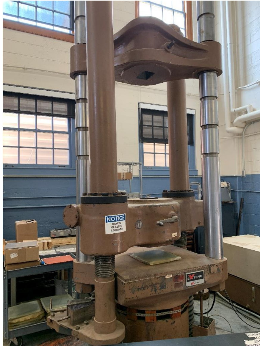
Figure 12: 400-kip Baldwin testing frame used for consolidation.
