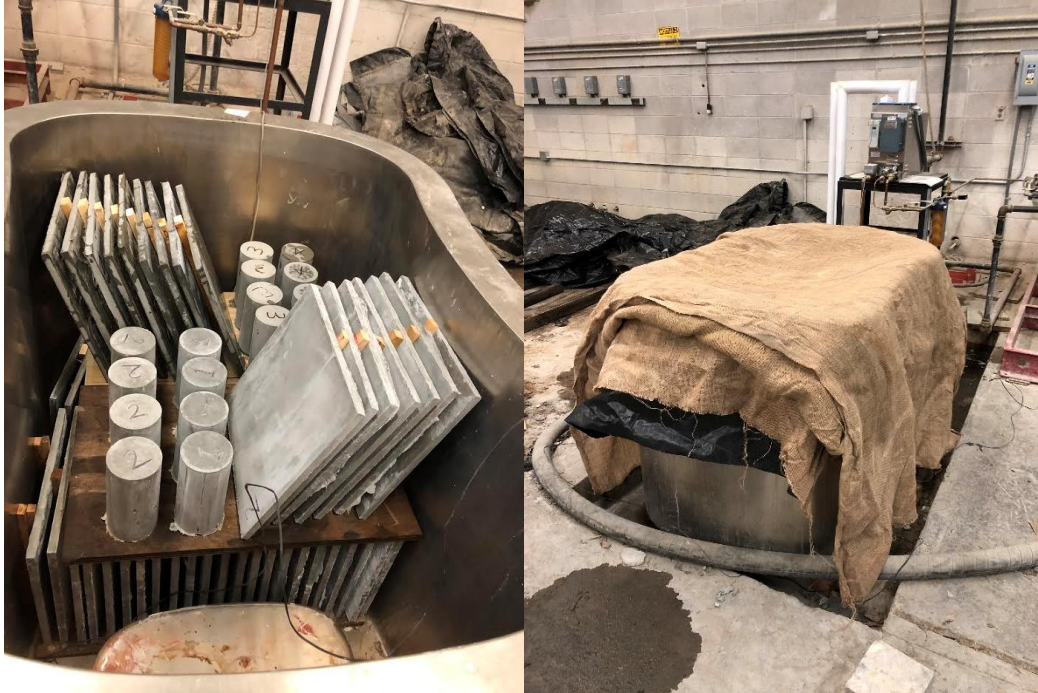
Figure 2: Insulated Japanese soaking tub with steam generator used to cure UHPC panels (left) and tub covered in visqueen and burlap insulation (right).
