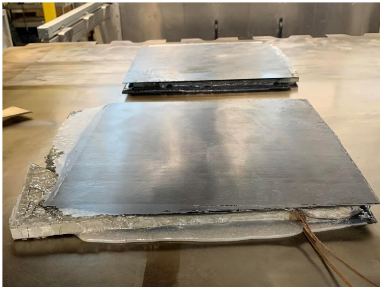
Figure 8: Issues with the sandwich panels following the first consolidation trial.
