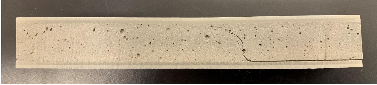
Figure 34: Typical concrete shear failure of the beams.
