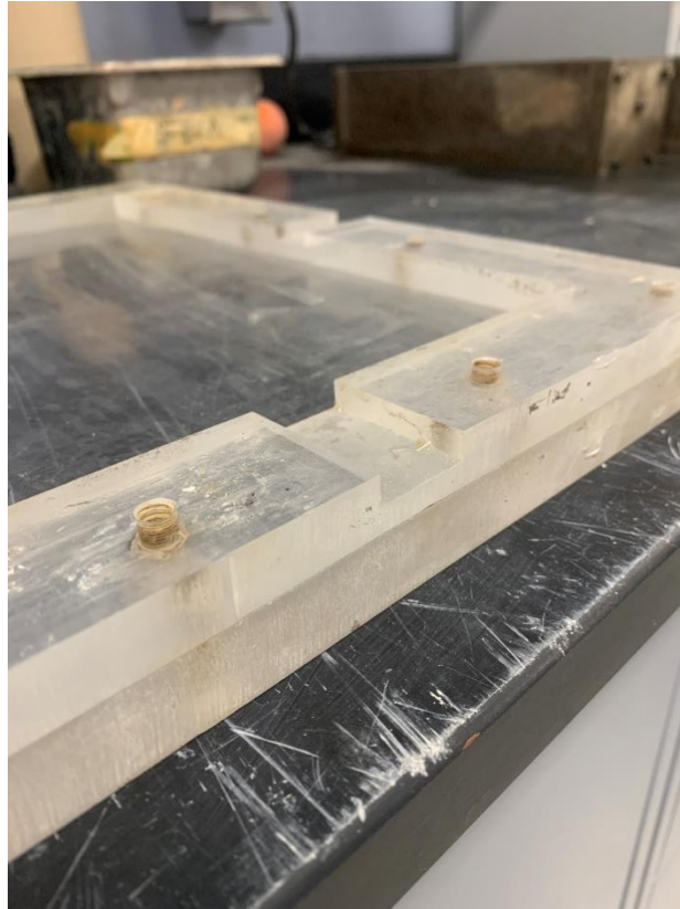
Figure 3: Small channels cut out of 5-sided UHPC panel mold.
