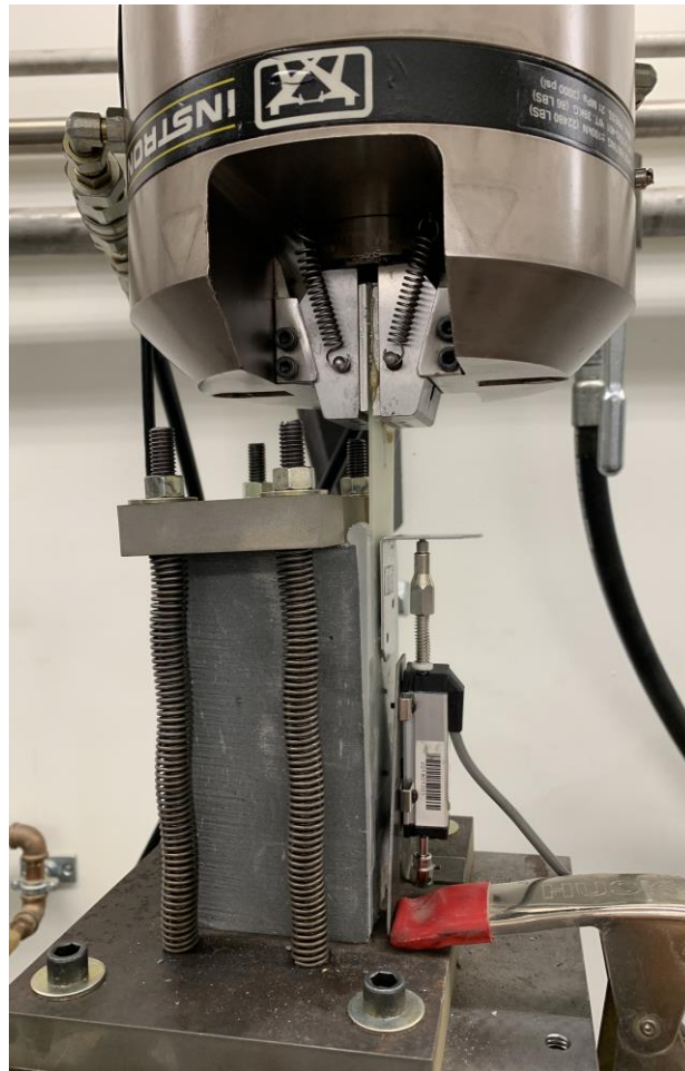
Figure 44: UHPC-thermoplastic single-lap shear test setup.
