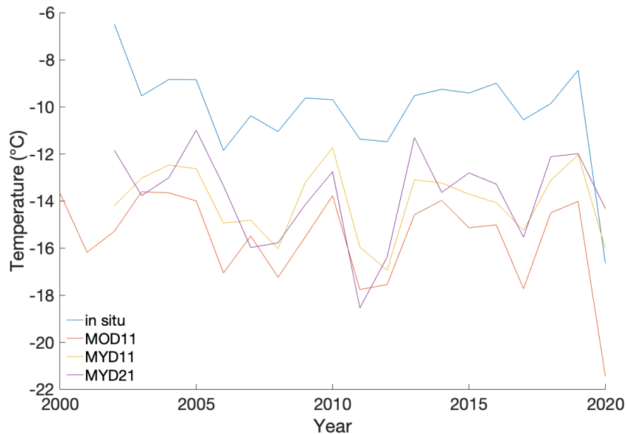
Figure 2.13. Mean annual MODIS and in situ temperatures at Divide. Results show a prominent cold bias in the remote sensing measurements (purple, yellow, orange lines) compared to the in situ measurement (blue line), but overall agreement in years of high vs. low temperatures.
