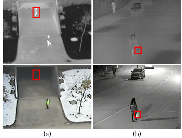
Fig. 1. Illustration of the complementary information between multi-modal images. (a) and (b) are two exemplar frames from RGB modality and thermal modality, respectively. As shown in the regions marked by the red boxes, obvious complementary information exists between the two modality images, which will benefit the subsequent tracking task.
