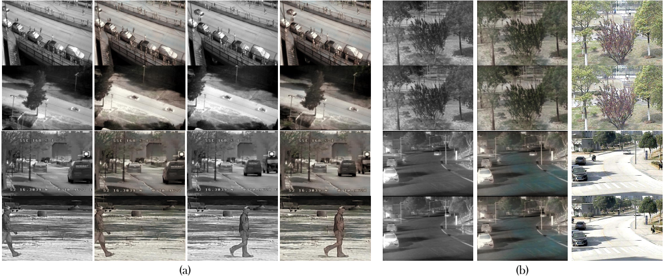
Fig. 10. More examples of our generated RGB images. (a) In each row, we present two pairs of RGB-T images spaced 30 frames apart in the same video; (b) The first column is original thermal images, the second column is synthetic RGB images, and the third column is real RGB images corresponding to the first column of thermal images.
