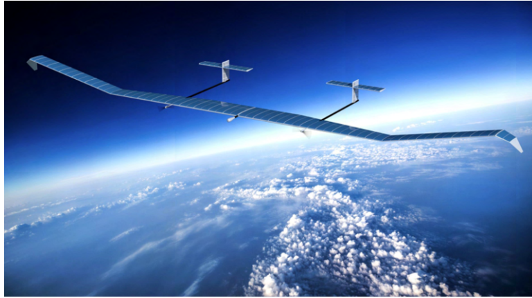
Figure 1.2: The Airbus ZephyrT high altitude pseudo-satellite. This is the larger of the Zephyr series of solar aircraft designed for military and commercial use [2].
