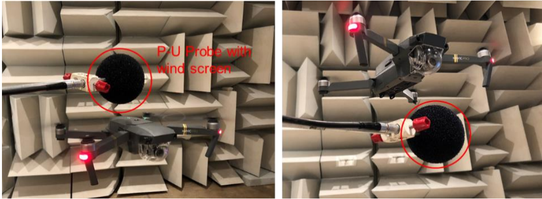
Figure 5.4 Particle velocity and sound pressure measured on imaginary box
