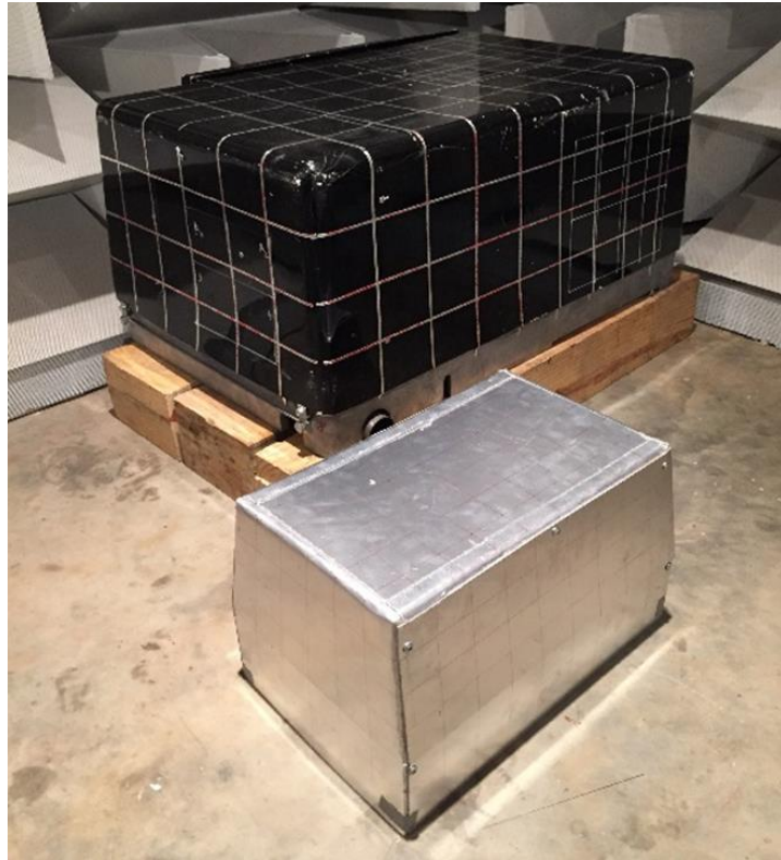
Figure 3.5 Generator set and half-scale model used for transfer function measurements
