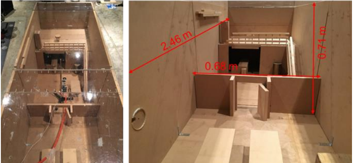
Figure 4.7 1/10-Scale model of bakery
