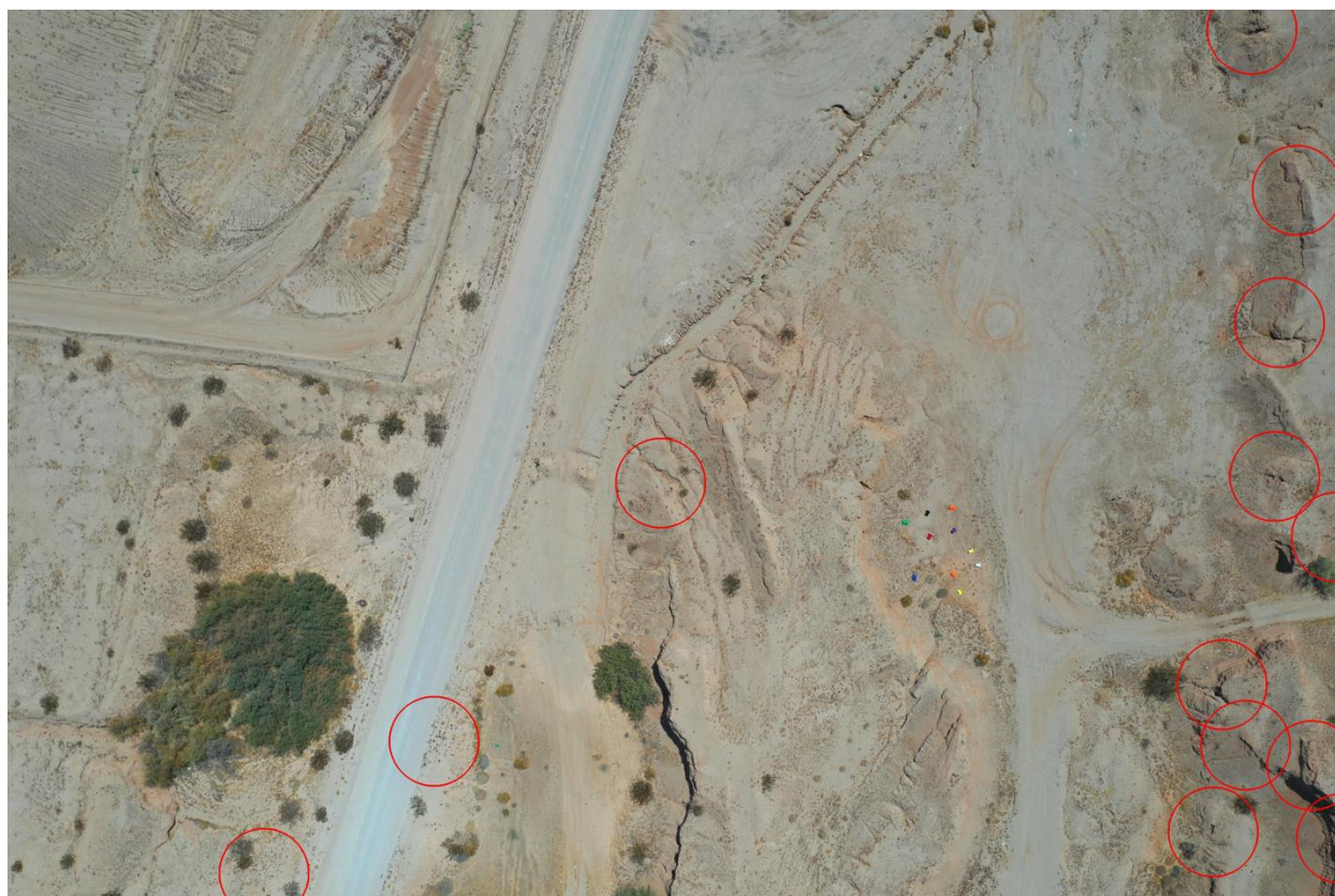
Figure 13. Flagged image captured by Mavic 2 Pro at 400 feet AGL. Target search color was purple. Loc8™ identified 13 as possible matches. Operator analysis of the flagged image showed that all 13 areas were false positive detections. The torso model with the purple garment was also in the image; however, it was not flagged by Loc8™ as a possible match.
