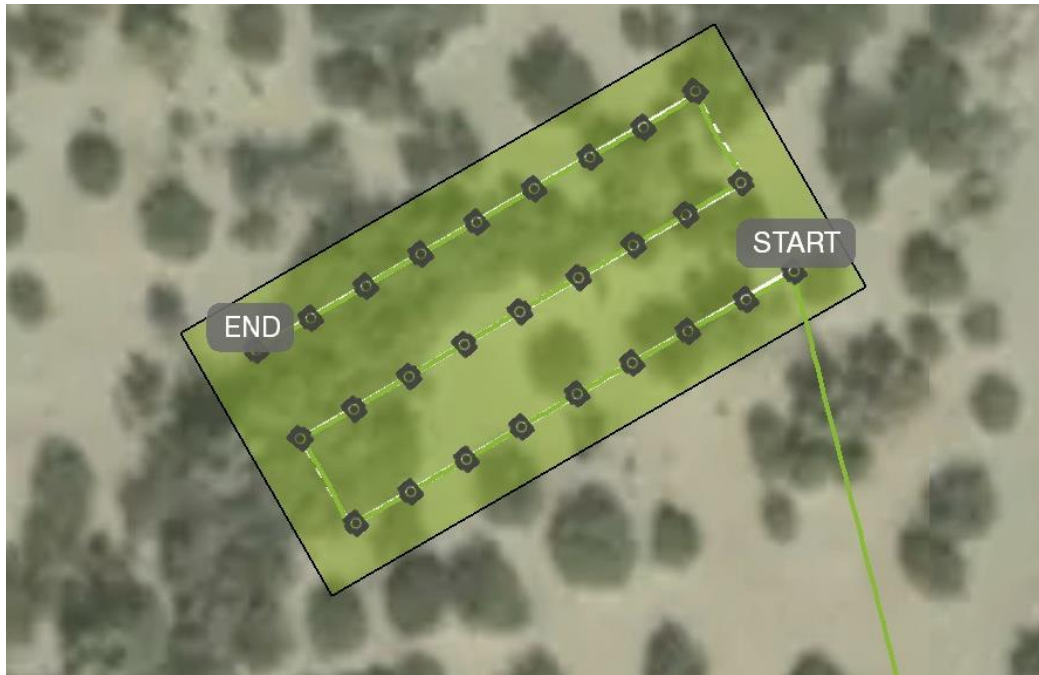
Figure 7. Screen capture of completed Mavic 2 Pro flight plan. The camera symbols indicate the location and the direction of the sensor when each image was taken.
