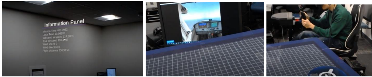
Figure 6. Augmented flight information visible in the space, cockpit view on a separate monitor, and VR simulator visible while wearing a HoloLens headset (from left to right).
