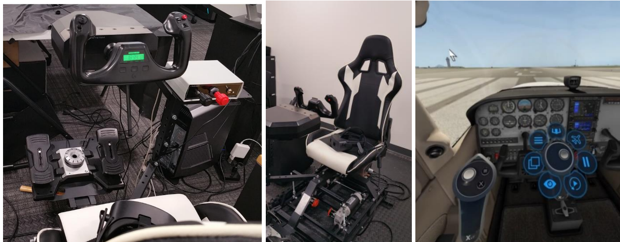
Figure 1. VR simulator controllers, VR simulator seat, and motion platform: X-Plane VR cockpit view (from left to right).
