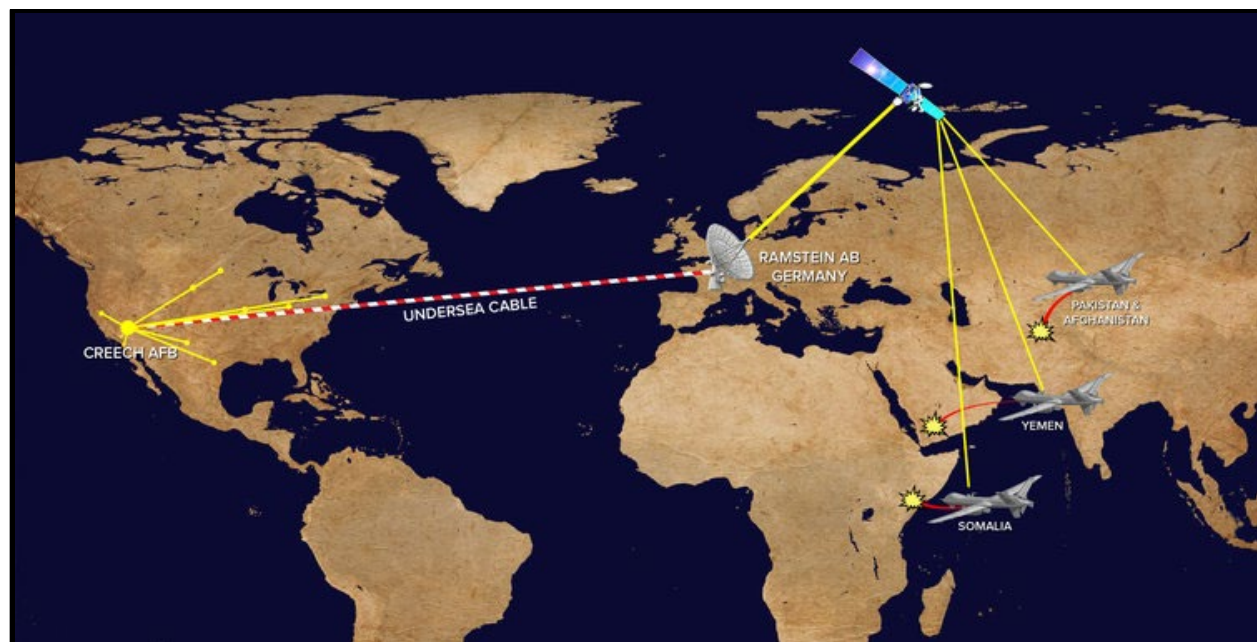
Figure 2. Hypothetical UAS satellite communications link. Adapted from Brownstein (2015).
